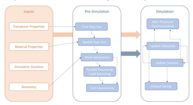
Figure 1 - EFIT-CompCell Functional Flow Block Diagram.
