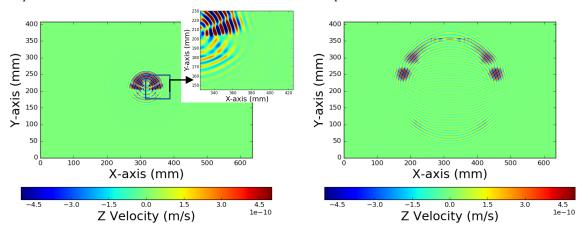
Figure 5-Z-component of Velocity for the smooth, outer surface of the panel at 25.28  $\mu$ s and 71.1  $\mu$ s for a pristine panel.
