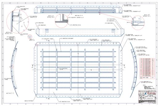
Figure 3 – Drawing of FAA fuselage test panel.
