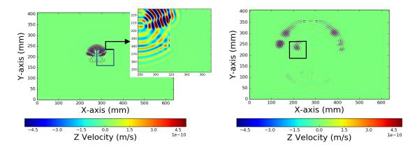
Figure 6 - Z-component of Velocity for the smooth, outer surface of the panel at time steps 25.28  $\mu$ s and 71.1  $\mu$ s for a Panel with a cut in the Y axis through the center stinger and skin.
