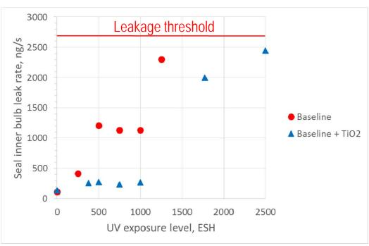
Note: Leak rates are steady state values at 23°C for fully compressed seals
