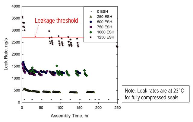
Leak rates for baseline seals also decreased as tests progressed, although magnitude of decrease was less than what was seen for seals with TiO2 additive
