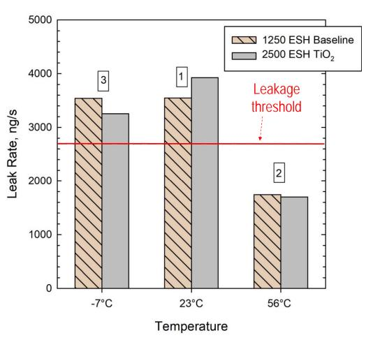
Note: Leak rates are steady state values for fully compressed seals. Test order noted by numbered boxes.
