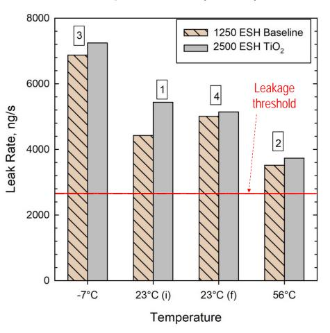
Note: Leak rates are steady state values for partially compressed seals (0.066 cm gap). Test order noted by numbered boxes.
