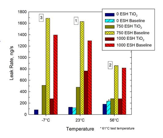
Note: Leak rates are steady state values for fully compressed seals. Test order noted by numbered boxes.
