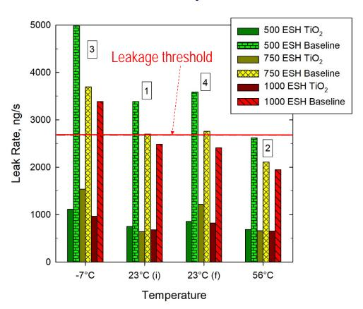
Note: Leak rates are steady state values for partially compressed seals (0.066 cm gap). Test order noted by numbered boxes.
