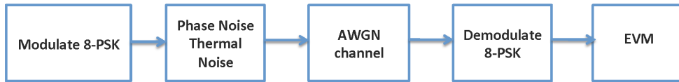
Figure 2. Block diagram of the measurement of EVM in the modulated and demodulated signals
