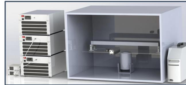
Conceptual drawing of multi-stress environmental test setup
