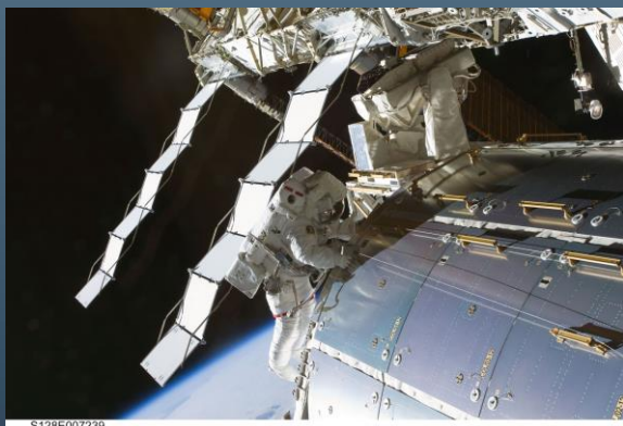
The space station's radiator system, which is a critical component of the active system, consists of seven panels (each about 6 by 12 feet)
