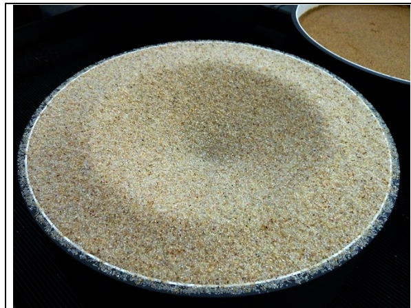
Figure 5. Photo of the crater formed into a target with a 3-cm layer of sand over a stronger substrate of bonded sand. The bonded sand is a darker color than the “regolith” sand, as seen in top right corner.
