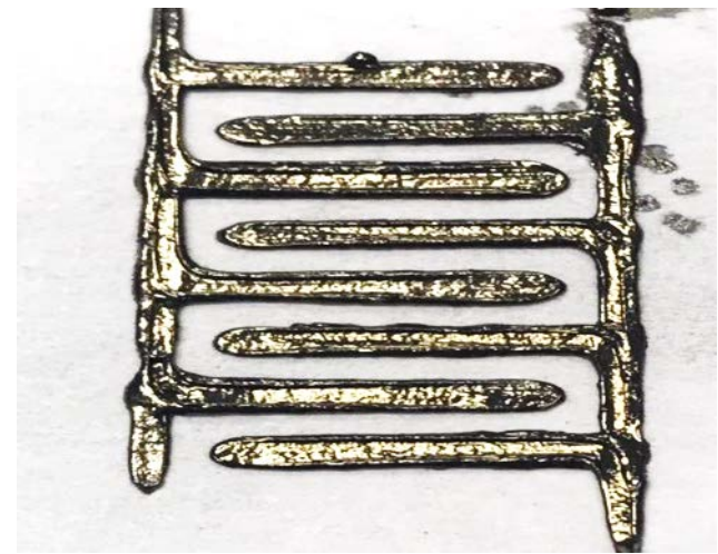
3D-Printed Al-Fe 3 O 2 Nanothermite Sintered CO 2 Sensor
