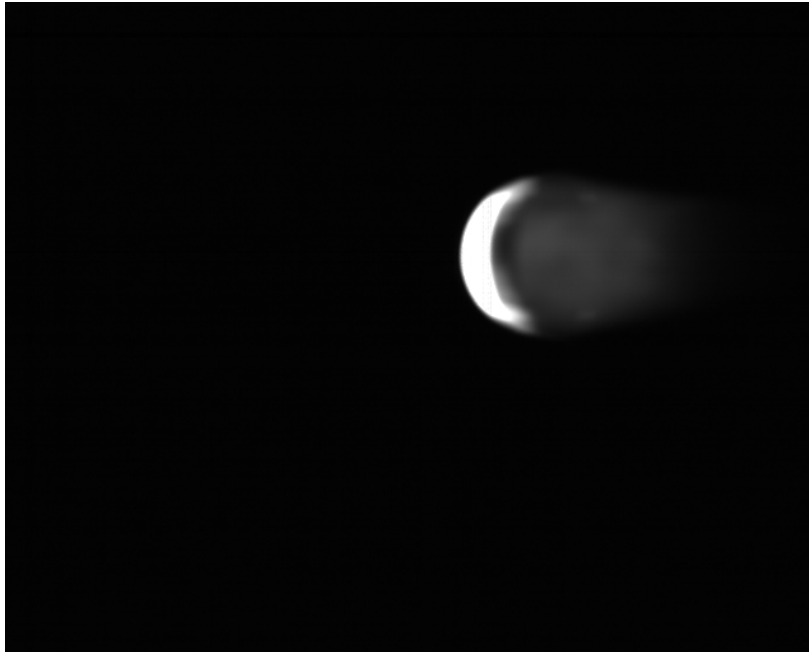
Figure 17. Afterbody IR picture for shot 2720. Stainless steel hemisphere at nominal test condition of 5 km/sec in 76 Torr CO 2 . Both helium plume cans seen in Figs. 10 - 11 were used for this shot.
