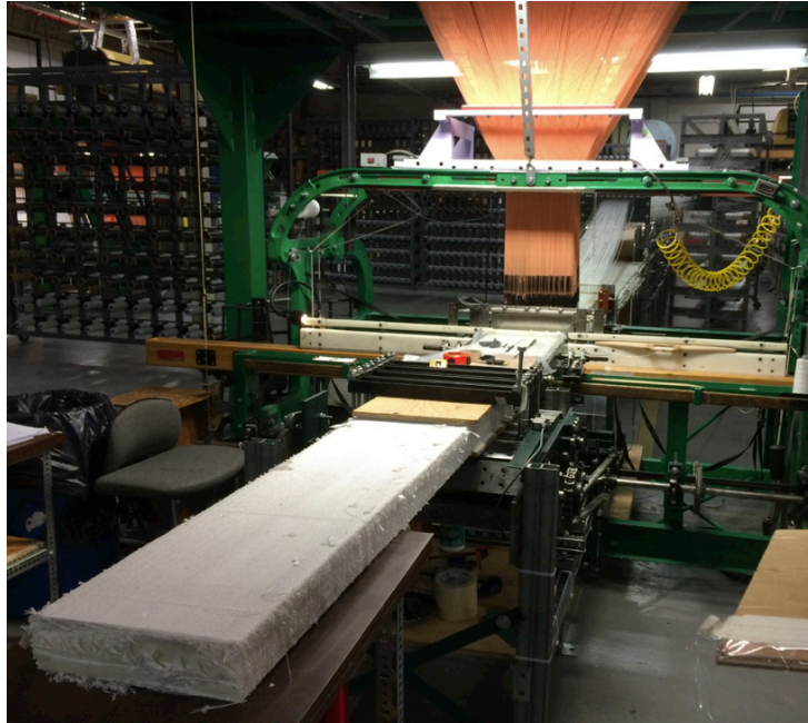
Figure 7. 3DMAT quartz preform weaving at Bally Ribbon Mills.
