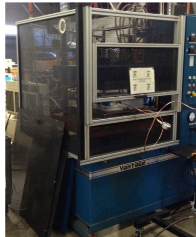
Figure 8b. Vessel installed a hydraulic press for cure.
