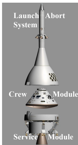
Figure 1a. Components of Orion MPCV.
