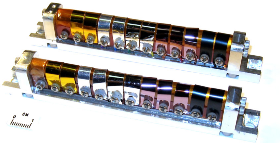
Figure 5. Pre-flight photograph of the two FSEE holders with the flight samples.
