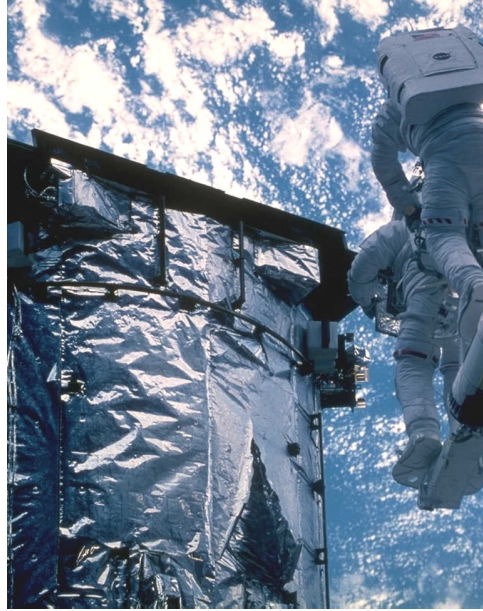
Figure 1. Example of cracking of the aluminized-Teflon FEB insulation on the HST after 5.8 years of space exposure (Ref. 2).
