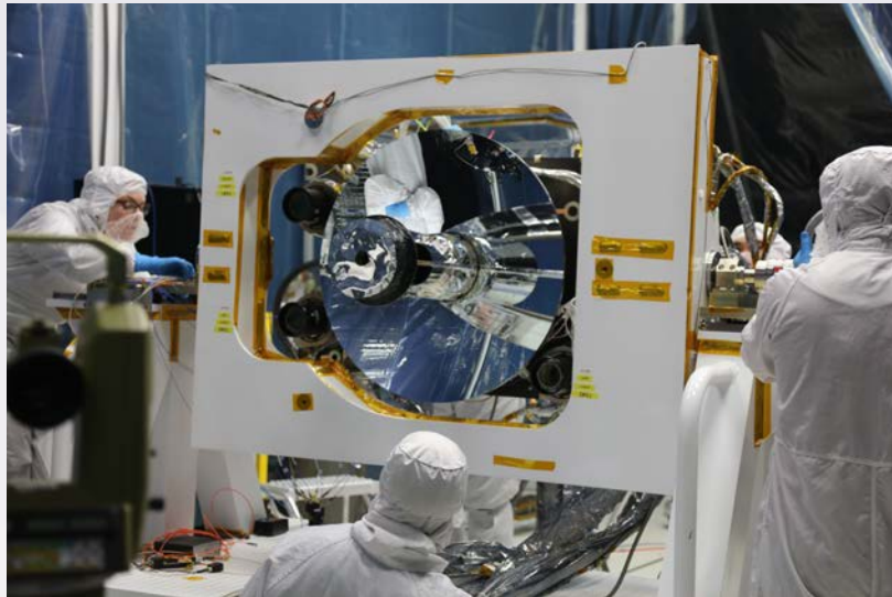
Global Ecosystem Dynamic Investigation (GEDI) optical bench installed in the GEDI Turnover Dolly. RTA (Receiver Telescope Assembly) and transmitter beam expanders seen
