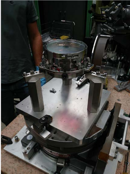
Chamber to perform interferometric testing of grism prototype under 150K
