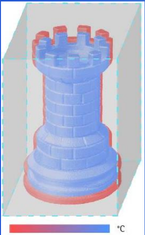
Cooling shrinkage behavior.
