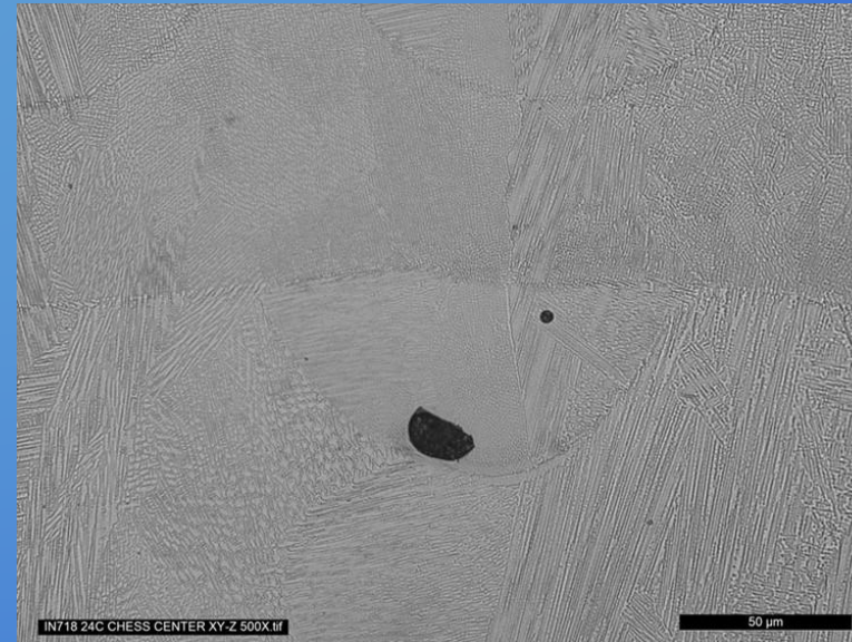
Shrinkage (keyhole) porosity in IN718 results from high laser power or fast scan speed.
