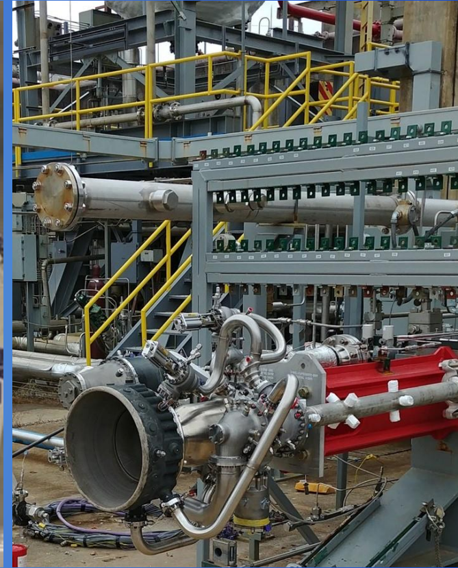
AMDE on the test stand at MSFC.
