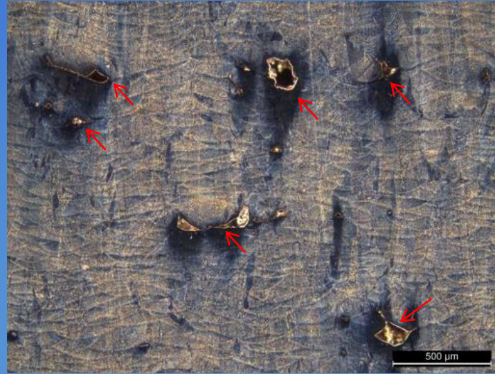
H-LOF defect from insufficient laser power (set point or attenuation).
