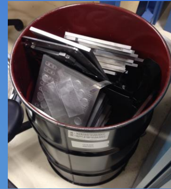
Spent build plates and oversized powder
