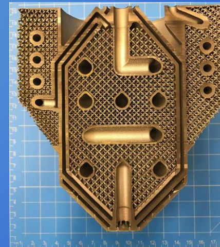
Cryo Heat Exchanger, Injector, Condenser
