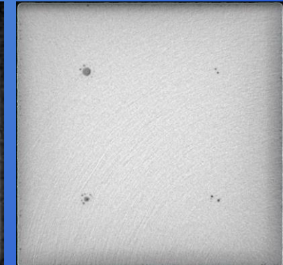
Known flaws in AlSi10Mg block. Left: Regular CT. Right: Micro-CT
