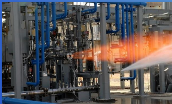
GRCop-84 AM Chamber Accumulated 2365 sec hot-fire time at full power with no issues
