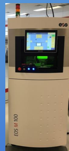
EOS M100 \varnothing 100x95 mm Power: 200 W Laser Diameter: 40 \mu m Material: Ti64, 316L, CoCr, Haynes 230. In-development: Haynes 282, JBK-75, HR-1.
