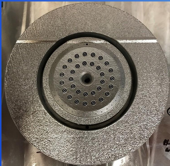
MET1 Injector V1 on EOS M290. Build time - $5.5k (55 hrs), Powder - $ 0.32k (5.82 kg), Saw - $0.2k, Plate resurface - $0.2k, Unsuccessful total - $6.22k. Successful total $6.22k. Total Cost $12.44k. 15 minute long simulation.
