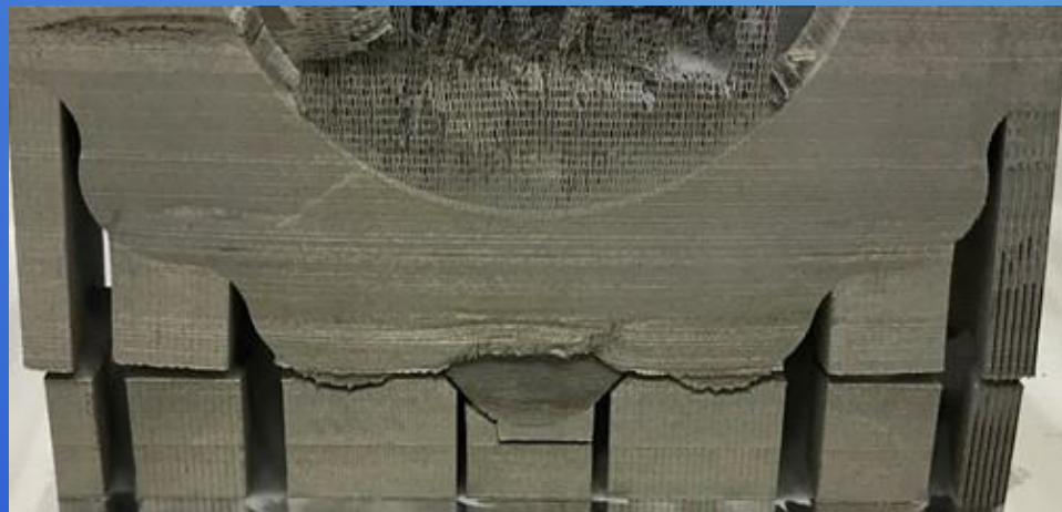
Residual stress induced failure.
