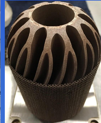
KSC O 2 Generator Cold-Head
