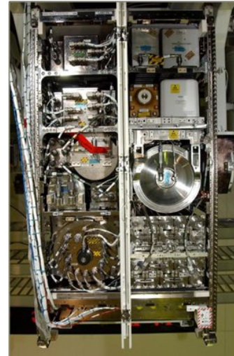
Water Recovery System (WRS) Racks 1 and 2 (Activation March 2009)
