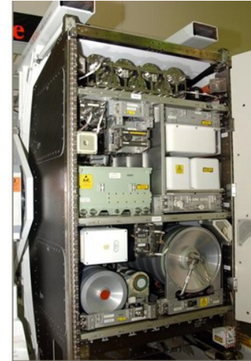
Water Recovery System (WRS) Racks 1 and 2 (Activation March 2009)
