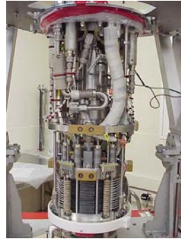
Hydrogen ORU without dome
