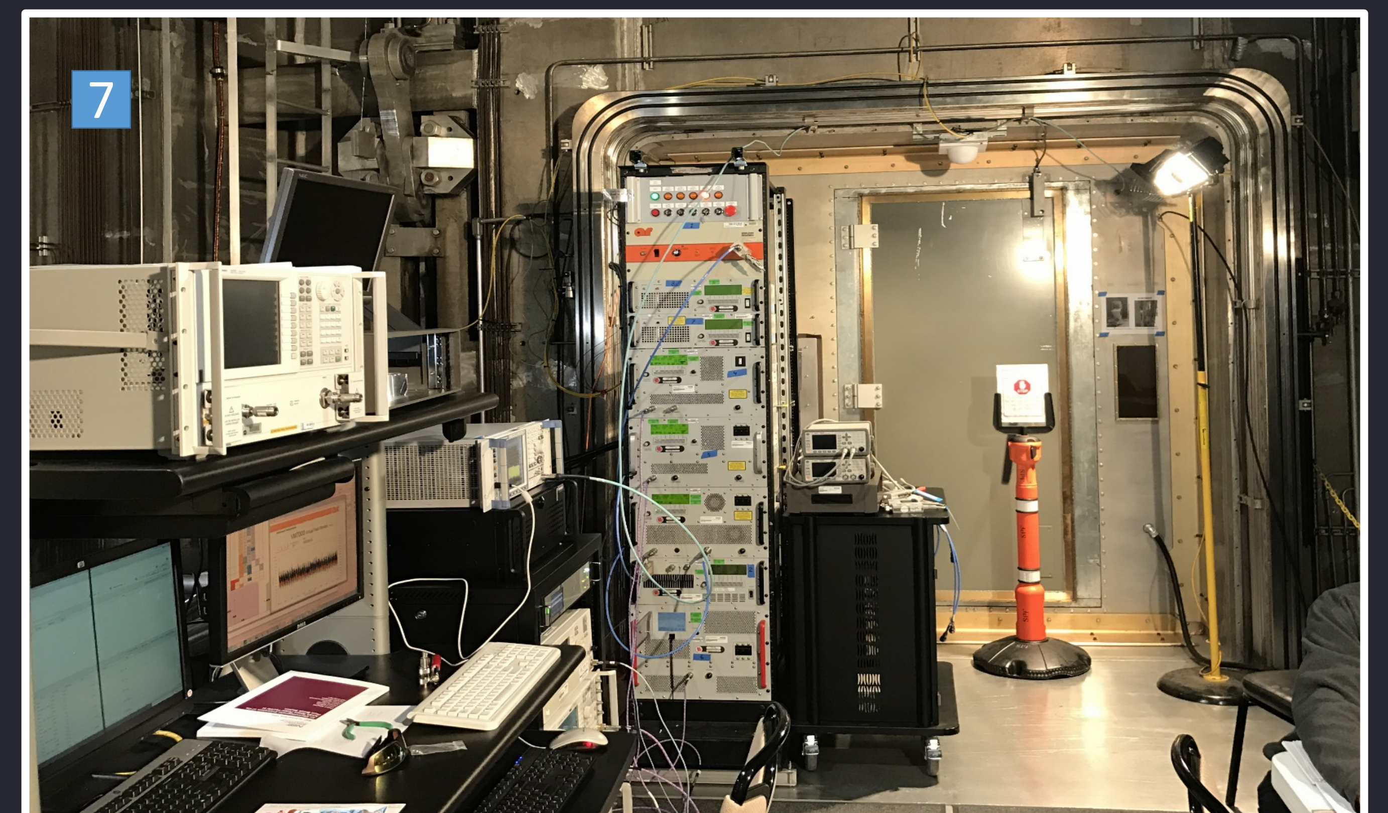
High-Power amplifiers just outside the chamber
