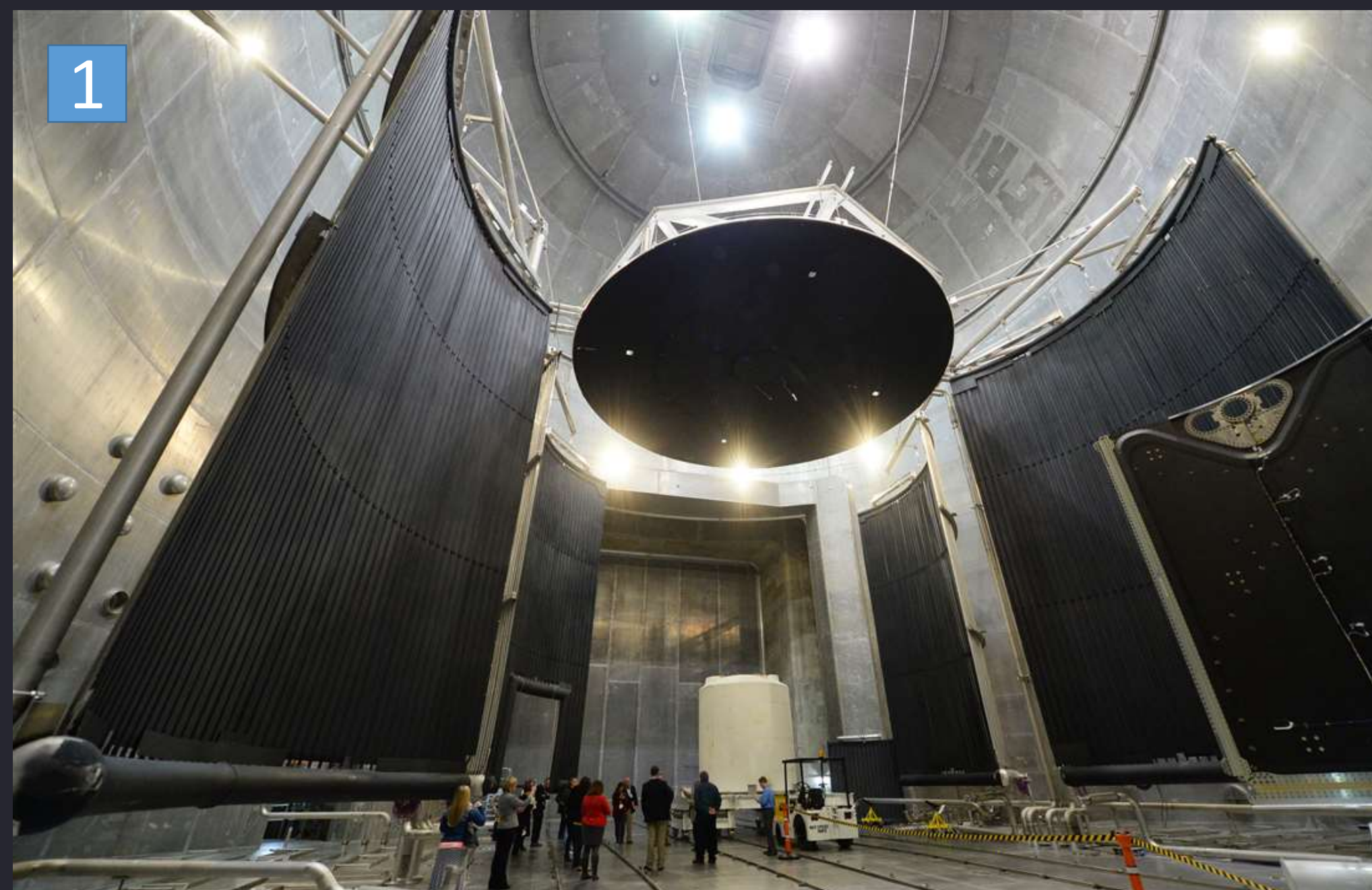
SEC is an electrically large (120' x 100') and electrically complex RF cavity
