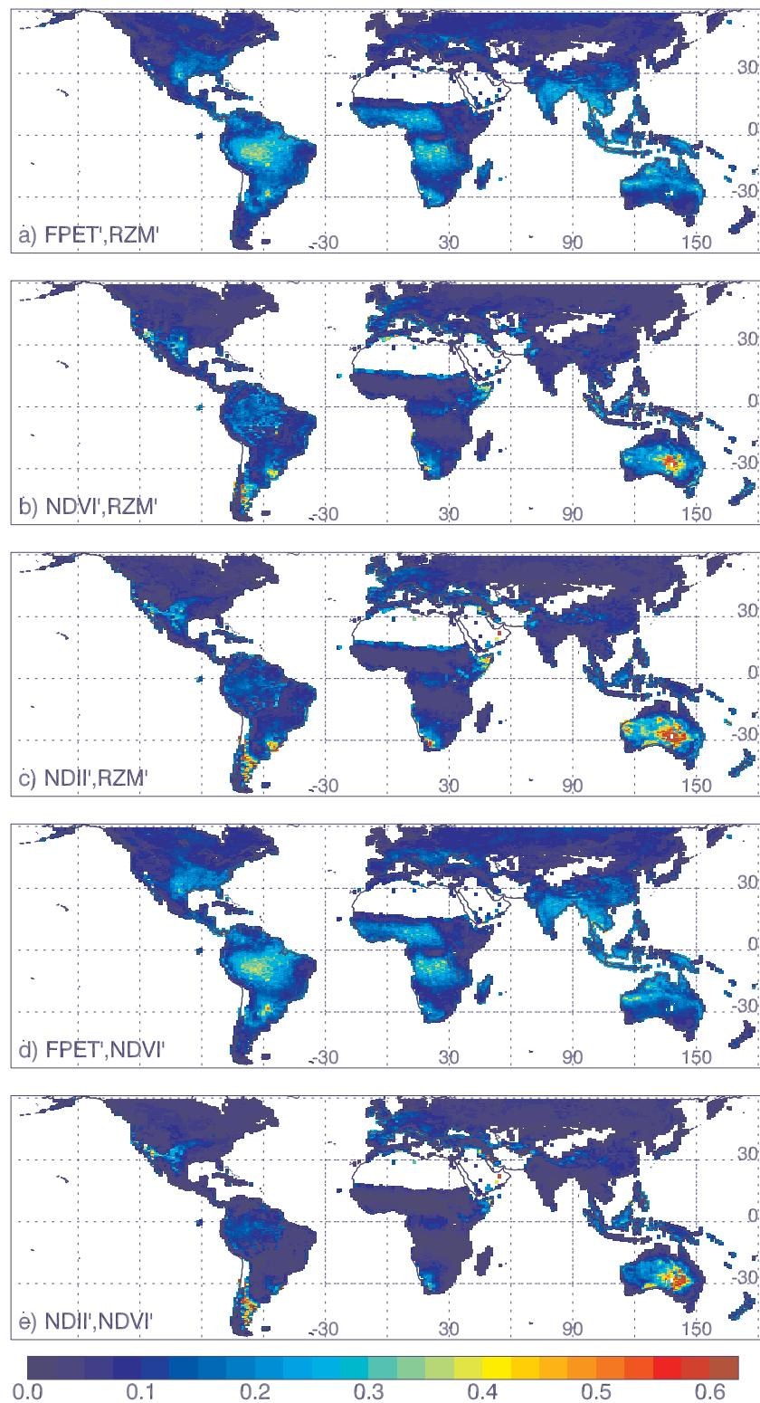
**Fig. B.8.** Standard deviations of the fitting residuals for different pairs of gridded drought indicators using Eq. (2); the first variable listed is the fitted parameter (fit by a scaled and shifted version of the second variable): a) FPET' fitted using RZM'; b) NDVI' fitted using RZM'; c) NDII' fitted using RZM'; d) FPET' fitted using NDVI'; e) NDII' fitted using NDVI'.
