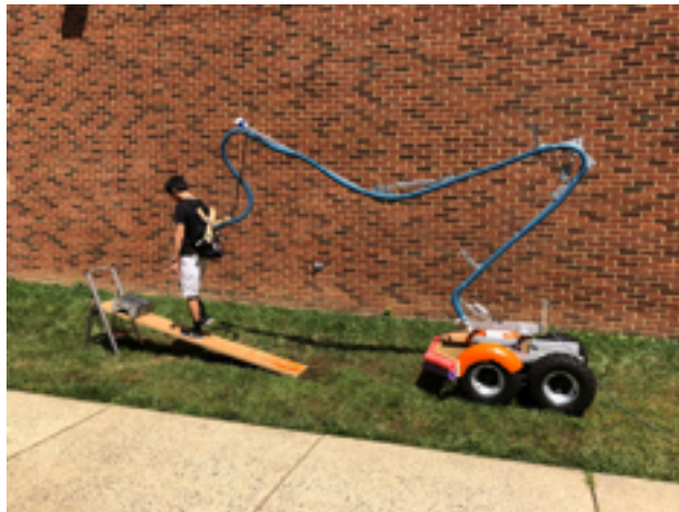
Figure 20: Actively controlled robotic umbilical handling mechanism
