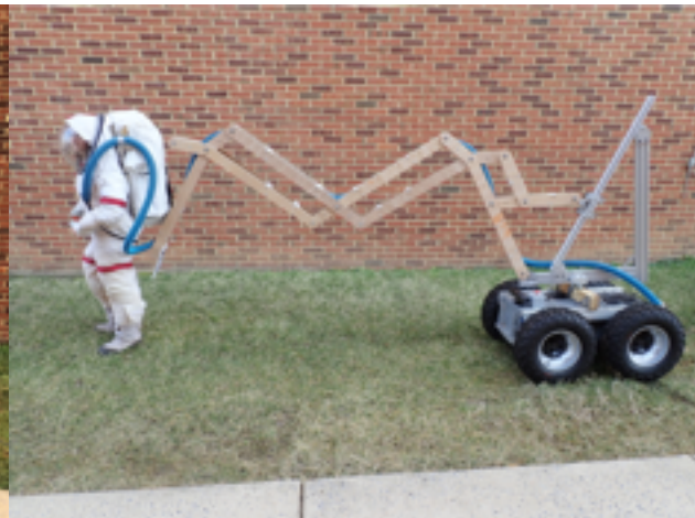
Figure 21: Passive pantographic umbilical handling mechanism
