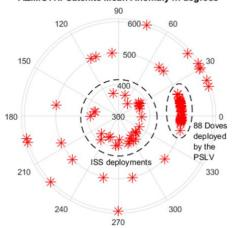
Figure 9: Orbital spread of the Planet satellites as analysed on Feb 18, 2017
