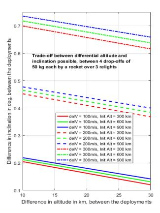
Figure 7: Differential altitude and inclination between consecutive satellites dropped off as a uniform spread, for different chief orbits and  $\Delta V$ .
