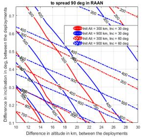
Figure 6: Time required for the first and last satellites to be positioned in perpendicular orbital planes after being dropped off by a Pegasus rocket deploying a four sat constellation.
