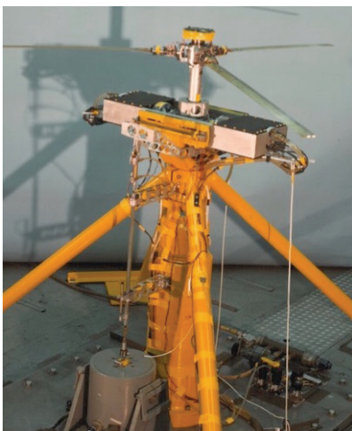
RDM for investigating coupled rotor-body aeromechanical stability in hover.
