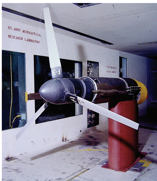
A 5-foot-diameter rotor test in the Army 7- by 10-Foot Wind Tunnel.
