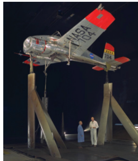
The X-14 in the 40- by 80-Foot Wind Tunnel with Crew Chief Cy Sewell and Ed Varette.
