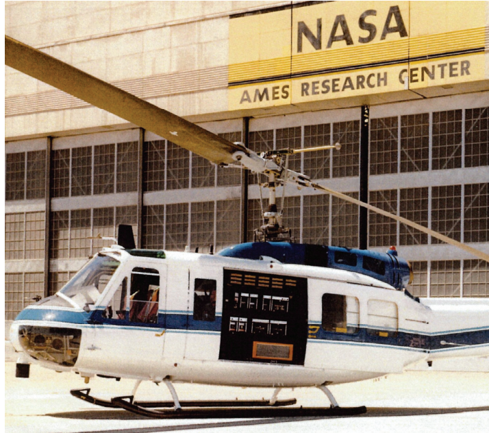
Air-cooled rack of V/STOLAND equipment.
