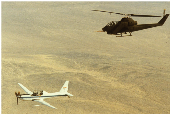
YO-3A aircraft gathering acoustic data while flying in formation with the AH-1G helicopter.
