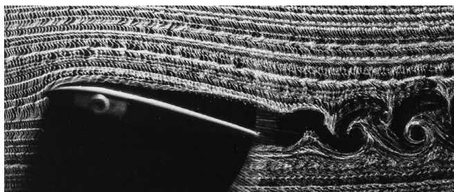
Hydrogen bubbles from a free-stream electrode.
