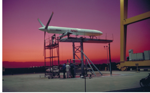
Early morning preparations for the XV-15 rotor hover performance test on the NASA Ames OARF, 1985.
