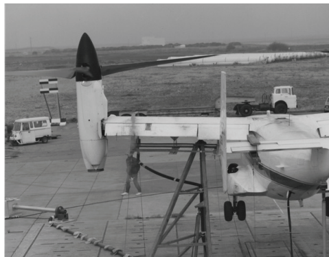
Flow visualization smoke test illustrating the chordwise flow near the wing tip.
