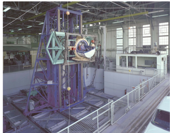
S.01 6-DOF motion simulator.
