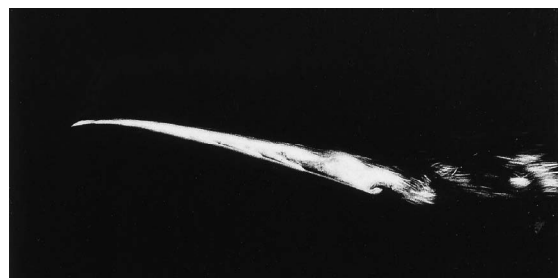
Hydrogen bubbles from surface electrodes.
