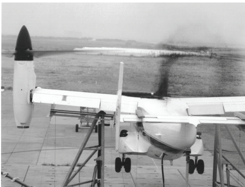
Flow visualization smoke test illustrating the fountain flow over the fuselage center.
