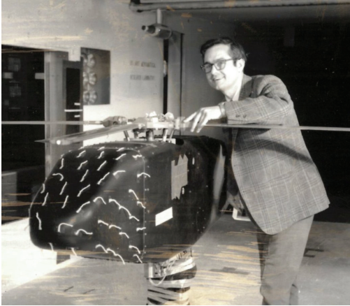
Dave Sharpe and the 7.5-foot Lockheed hingeless rotor model in the Army 7- by 10-Foot Wind Tunnel.
