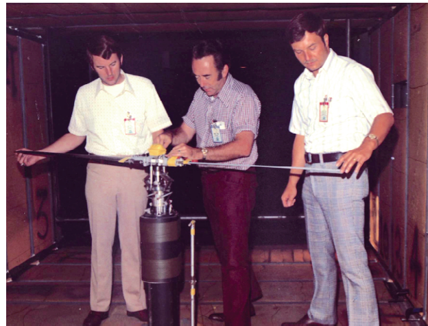
Don Boxwell, Bob George, and Fred preparing to test a UH-1H rotor in the acoustically treated 7- by 10-Foot Wind Tunnel.
