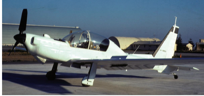
The FBI YO-3A aircraft after repainting and acoustic modifications.
