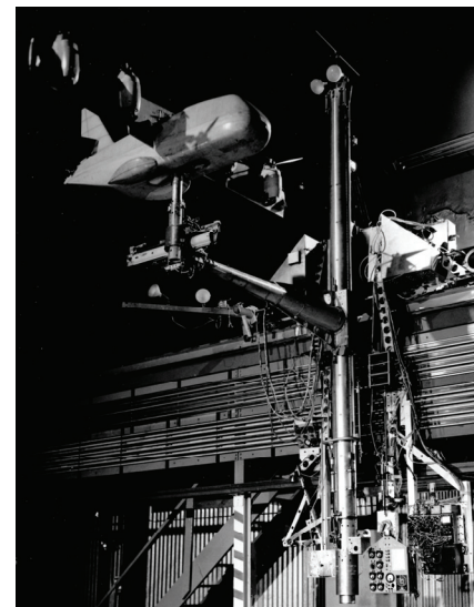
The XC-142 tiltwing VTOL aircraft model mounted on the Princeton University Long Track.
