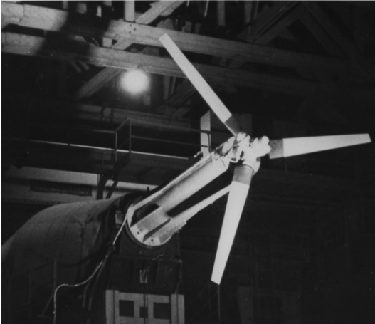
Hover performance test of a 13-foot-diameter rotor mounted on the AFAPL propeller test stand.
