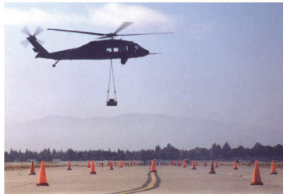
UH-60A with external slung load performing ADS-33 lateral reposition maneuver.
