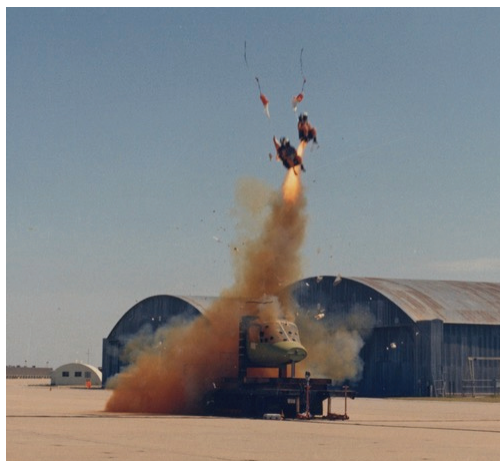
Simultaneous static test firing of XV-15 ejection seats.
