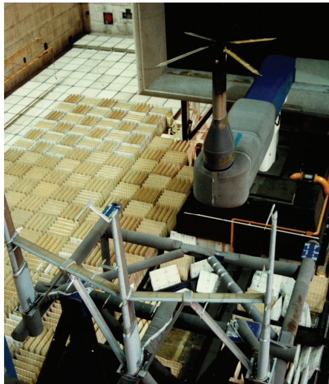
Noise testing in the DNW wind tunnel using the Boeing rotor.
