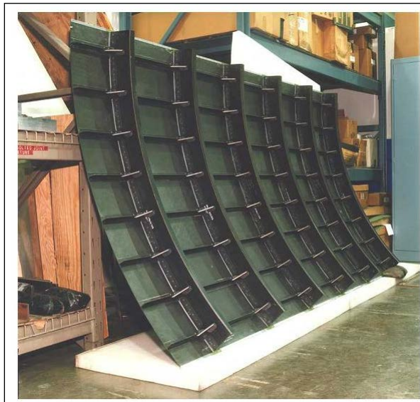
Figure 6.3-1: High-Temperature IM-7/PETI-5 Skin Stringer Panel (6'x10')
