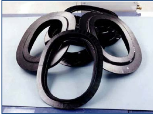
Figure 4.5-4: Completed Braided and Woven Window Frames
