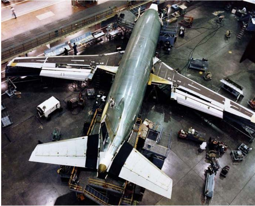
Figure 4.2-11: Advanced Horizontal Stabilizer Installed on B-737 for Airline Service
