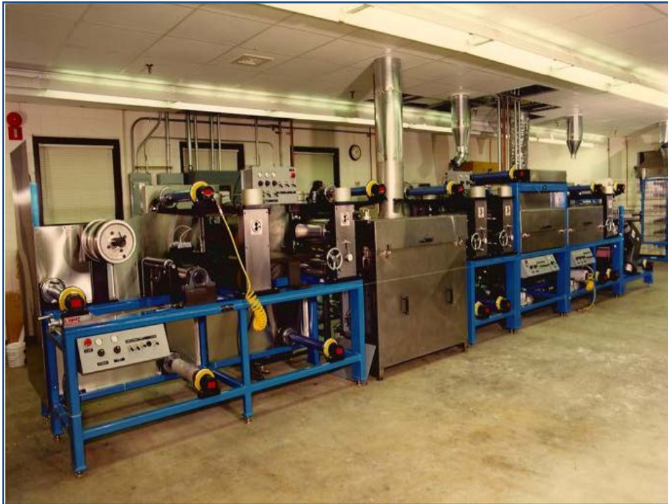
Figure 12.4-1: Modular Horizontal, Automated Prepregger Installed at LaRC
