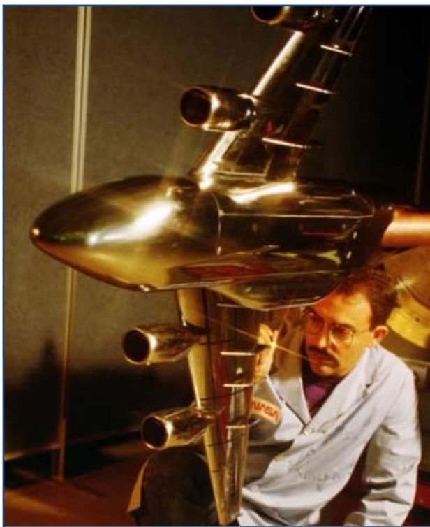
Figure 2.4-1: A High-wing Military Transport Model in Wind Tunnel at NASA Langley Research Center
