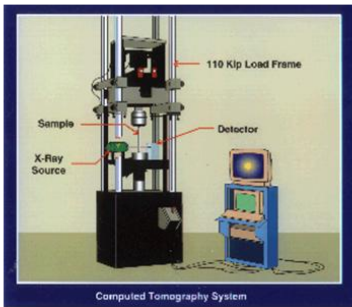
Figure 14.2-4: QUEST – Quantitative Experimental Stress Tomography system. This breakthrough system achieved its first image February 28, 1992. An example of a static image of a honeycomb is shown. The system can image the geometric distortion that occurs during loading or fatigue.
