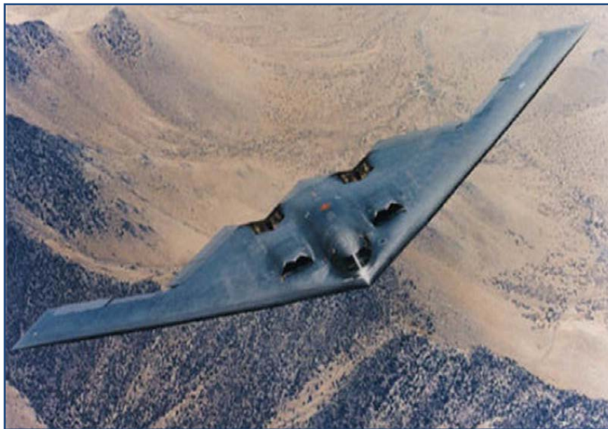
Figure 2.3-3: B-2 Primary Structure is Almost All Composite Materials
