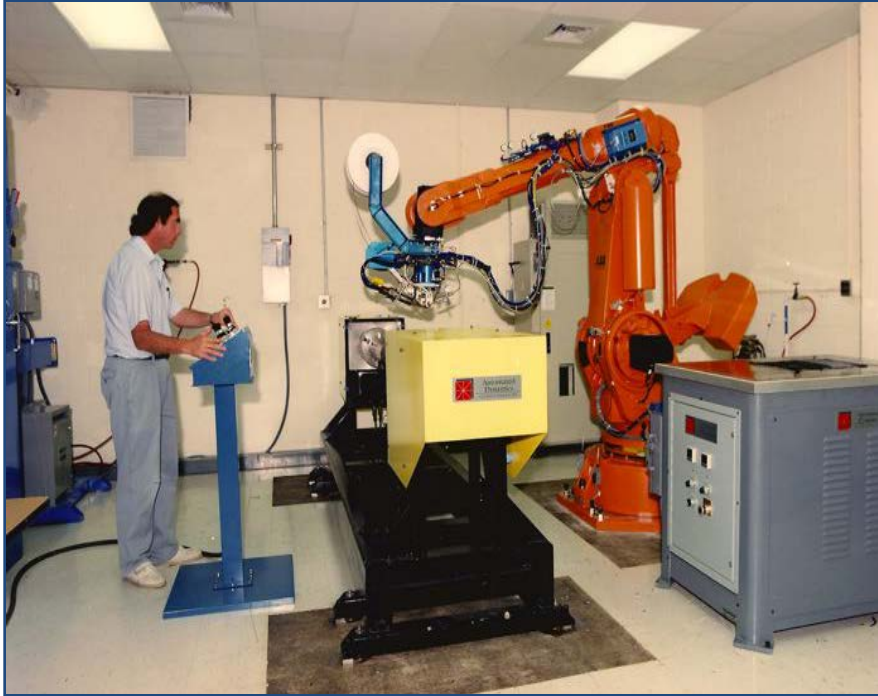
Figure 12.5-2 Photograph of the Heated-head Automated Tow and Tape Placement Robot Installed at LaRC.
