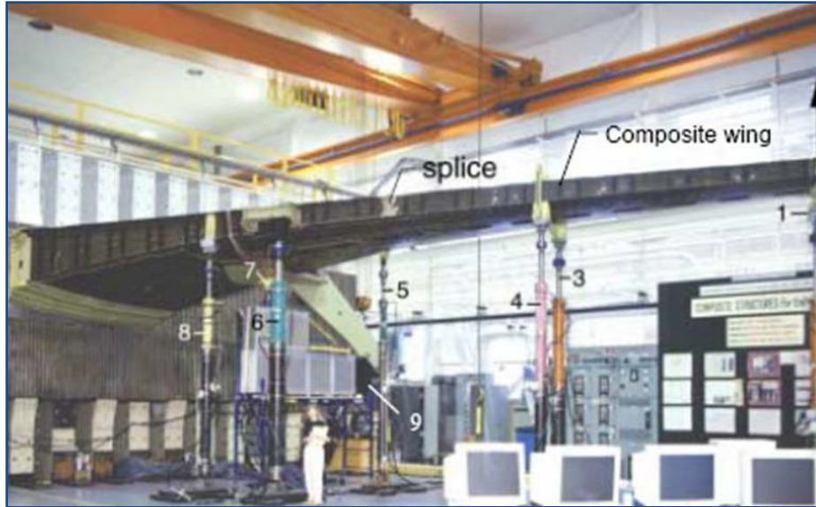
Figure 4.5-16: Semi-span Wing Prior to Testing at NASA Langley
