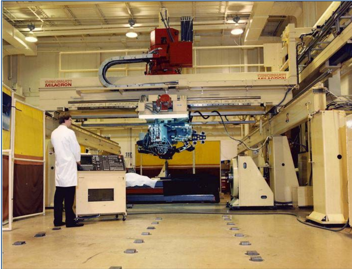
Figure 12.5-1: Accudyne ATP Heated Head and Controls on a Cincinnati Milacron Overhead Robot
