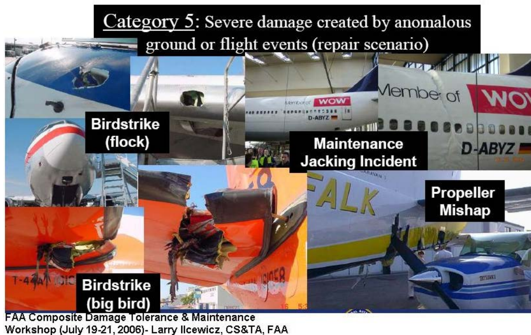
Figure 15.1-4: Examples of Category 5 Damage to Aircraft
