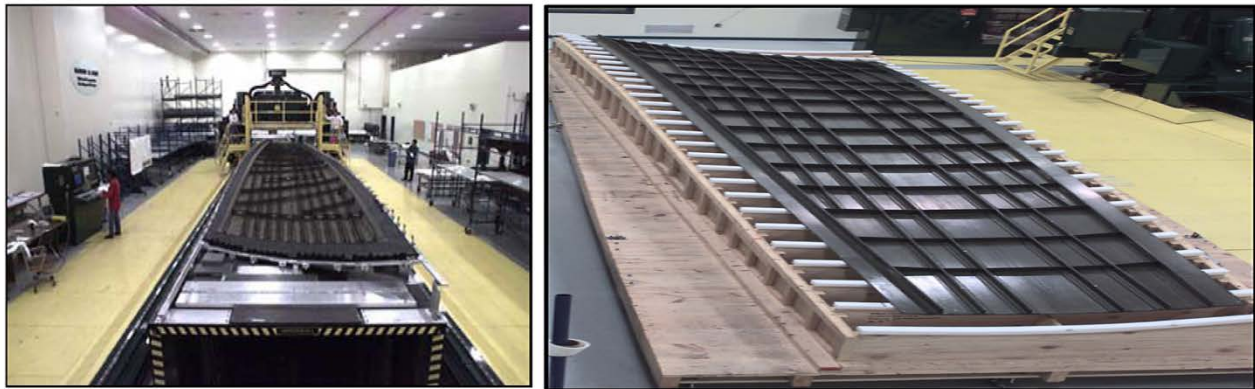
Figure 4.5-12: NASA's Advanced Stitching Machine with a Lower-stitched Wing Cover for a 42-ft. Span Structural Test Wing During Stitching (left) and Completed S/RFI Wing Panel (right). Located in the Marvin B. Dow Stitched Composites Center.
