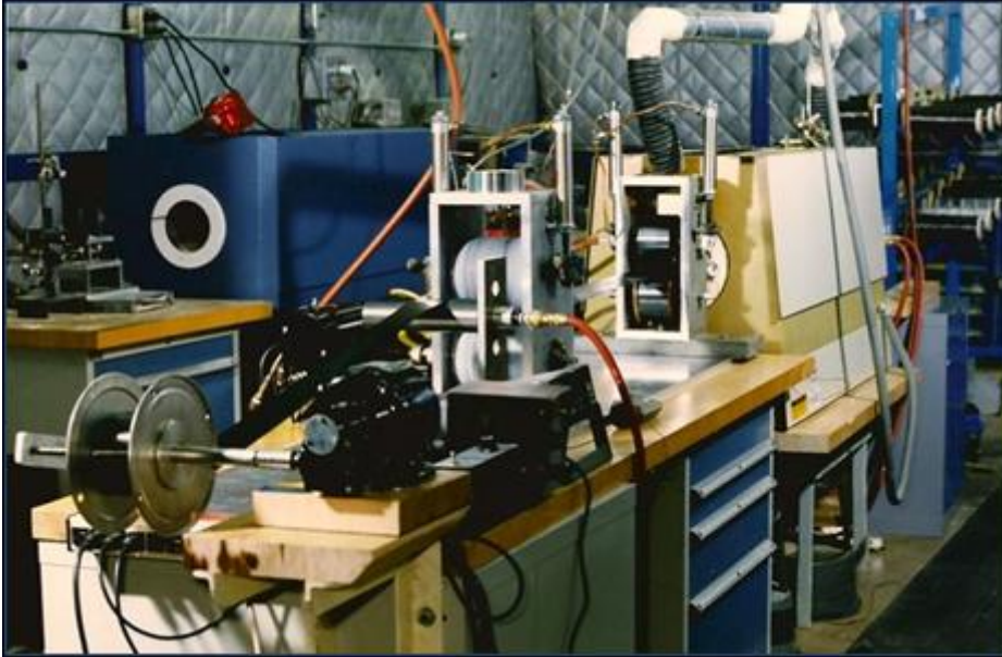
Figure 12.8-3: Photograph of the Ribbonizing Line Installed at LaRC in Building 1293C
