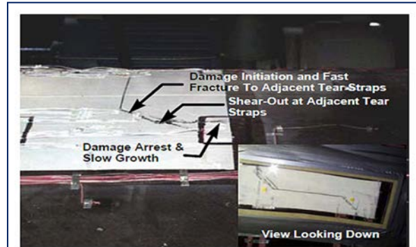
Figure 6.3-16: Photograph of Failed Fuselage Panel
