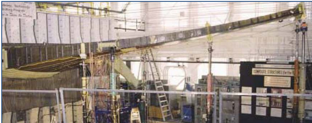
Figure 4.5-18: Deformed Semi-span Wing Test Article Loaded To 95% of DUL
