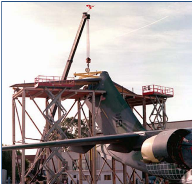
Figure 2.4-2: C-17 Horizontal Tail Redesigned Using Composite Materials
