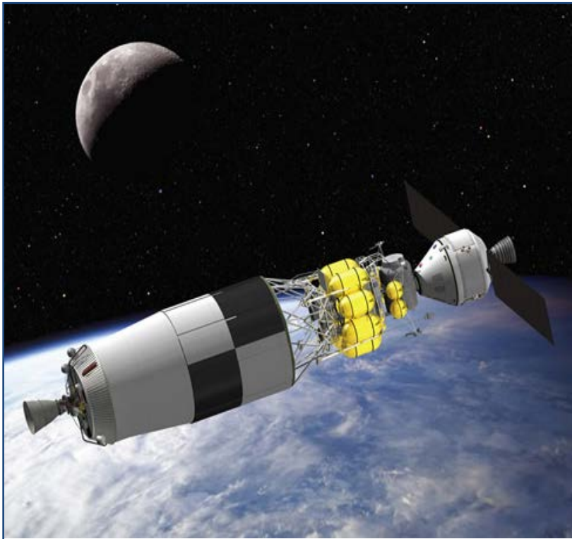
Figure 9.4-2: Concept Image of the Ares V Earth Departure Stage in Orbit, Shown with the Crew Exploration Vehicle Docked with the Lunar Surface Access Module (NASA/MSFC)
