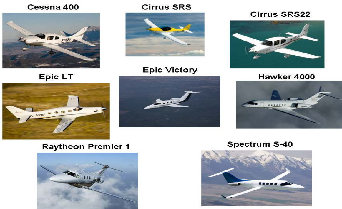
Figure 2.2-1: General Aviation Aircraft that have a Significant Amount of Composite Materials in Airframe
