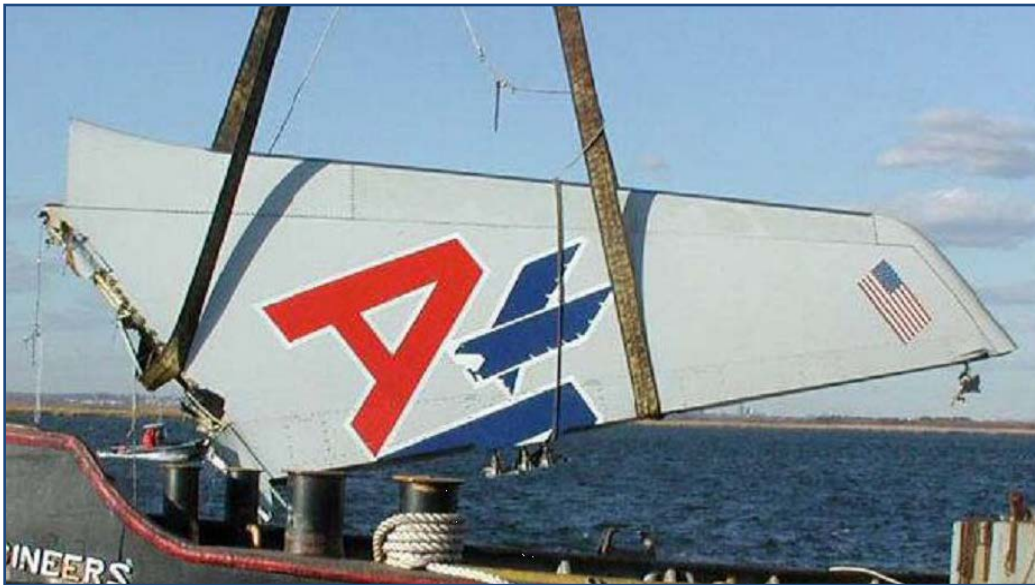
Airbus 300-600R Vertical Tail Plane (VTP) Recovered American Airlines Flight 587
