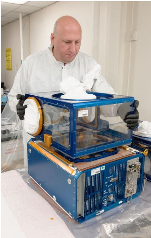
FIGURE 2 MICROGRAVITY HABITAT FOR MICE (CREDIT NASA)
