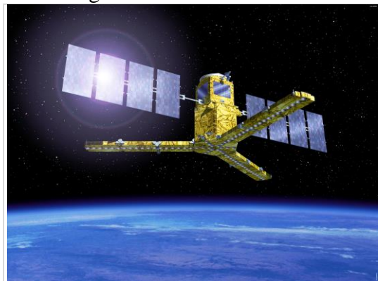
Figure 3: ESA SMOS mission satellite. A Y-shaped antenna array facing the earth, consisting of three equal arms separated from one another by 120^\circ . The satellite is shown above the rim of the earth, and is also equipped with two large solar arrays extending from a central hub which itself extends above the antenna on the non-earth-facing side.
