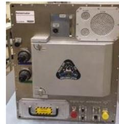
printer filament to create new tools and materials. The demonstration uses control plastic recycled multiple times to create parts to be tested for quality back on Earth. The Refabricator was placed into service on ISS in early 2019.
