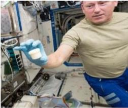
Inc. (MIS). The samples were fabricated using Fused Deposition Modeling (FDM) of polymers and were returned to NASA's MSFC where they underwent extensive testing, along with the ground-printed controls, to assess if there were any differences in the parts produced in microgravity from those manufactured on earth. Results indicated that there is
