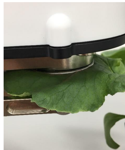
Figure 2 : The leaf is clamped to allow for carbon dioxide, light response and light-fan response measurements to take place.
