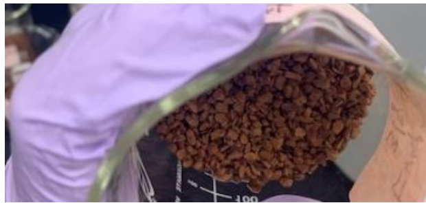
Figure 6. Image of “free water” in the beaker. This water has not yet been absorbed by the arcelite, which indicated that the arcelite is saturated with water.
