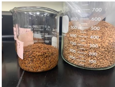
Figure 5. Comparison of dry arcelite (right) to the test arcelite (left) after three days.
