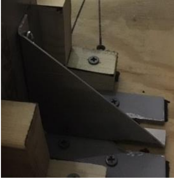
Figure 12. Stiffener to backside of the mount. Image Credit: Giovanni Campos, NIFS Intern.
