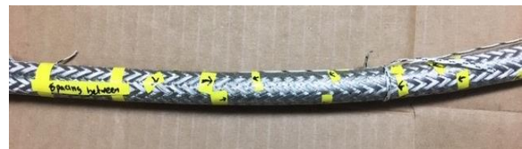
Figure 1. Quality Check of the Flex Hose.
