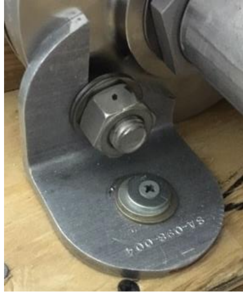
Figure 13. Extra Bracket attached to the Flange. Image Credit: Giovanni Campos, NIFS Intern.
