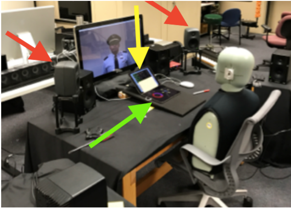
Figure 1. Experiment location with loudspeakers and touchpad displays. The numerical score (not shown) for the bias conditions is located at center bottom of the large display with the check pilot.
