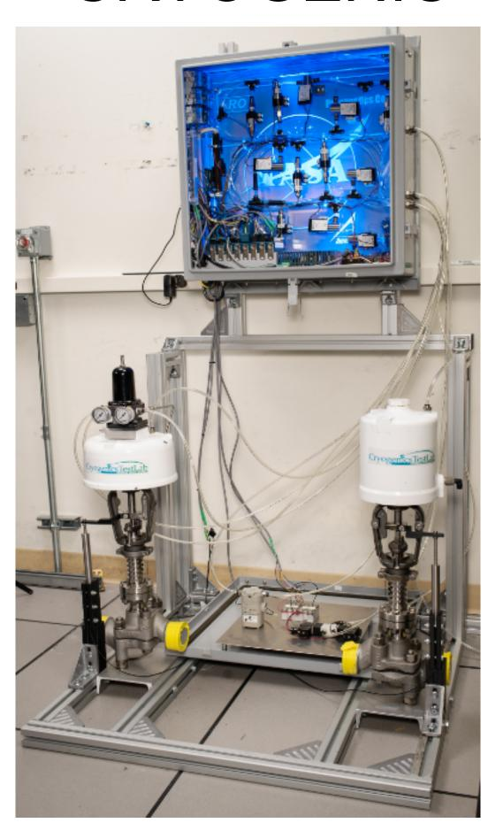
The Cryogenic valve testbed injects controlled faults into the cryogenic fuel valve system in order to accurately determine failure behavior. Data obtained from such experiments is useful development algorithms determining remaining useful life and end of life for the valves in the fuel loading system. Additionally, the diagnostic and prognostic methods developed with this system can potentially be used for future missions to help manage safety or degradation in a similar system.
