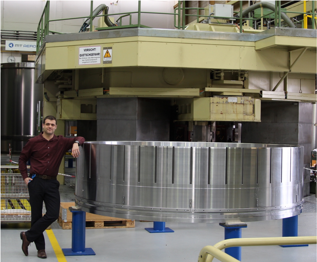
Figure 2. 10-ft. diameter ISC mandrel and forming equipment seen behind the mandrel. (Image used with permission from MT Aerospace)
