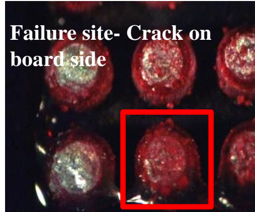
(a) Failure on board side
