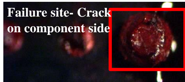
(b) Failure on component side
