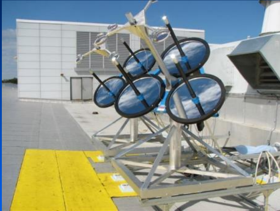
2 m 2 of collectors on solar tracking drive (NASA KSC)
