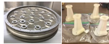
Design Database Development Printed Life Support System (LSS) Retaining Plate (Left); Urine Funnels (Right)
