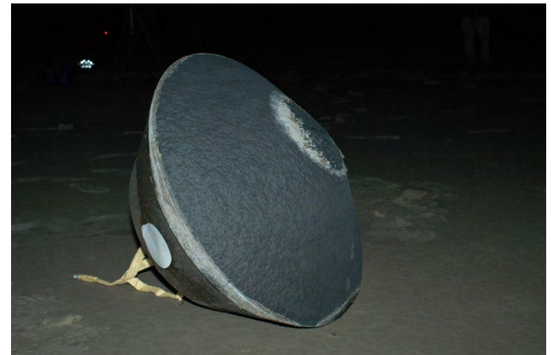
Stardust single piece, seamless heatshield
