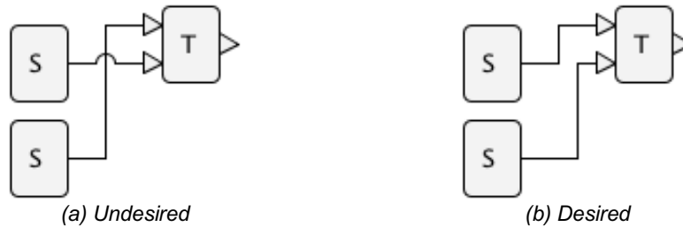
Figure 5.14. Link overlapping is avoided by reordering input pins
