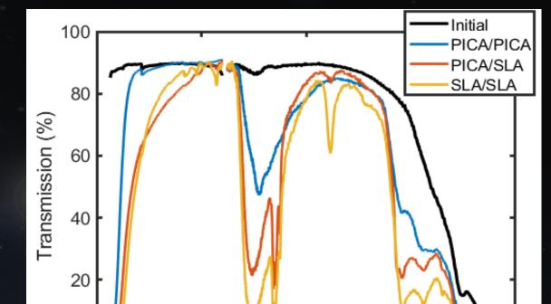
High-temperature sapphire rod coupled to mini-spectrometer configuration was tested using NASA Quartz Lamp source. Plots shown give effect of sapphire rod on system response and a representative calibration using integrating sphere. (Cruden & White)
