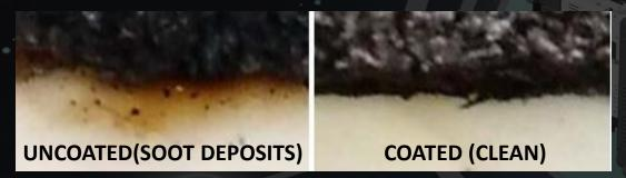
Evaluating space-qualified coatings (low-char Silicone, NuSil CV-144, Teflon, etc.) for window contamination control. First tests run: demonstrated concept in lab when low-char RTV protected glass from contaminating deposits. Characterized reflectance/ emittance effect of NuSil-coatings on PICA
