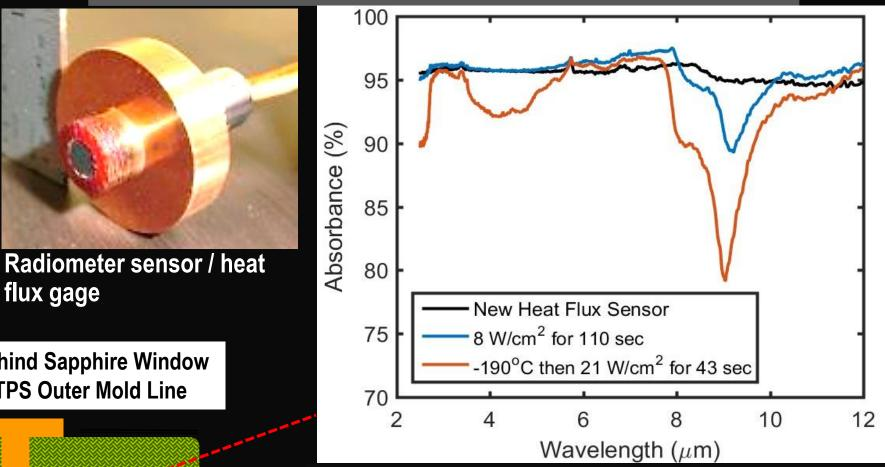
Coating degradation after aggressive thermal cycling / thermal shock but not from nominal test( Miller & White)
