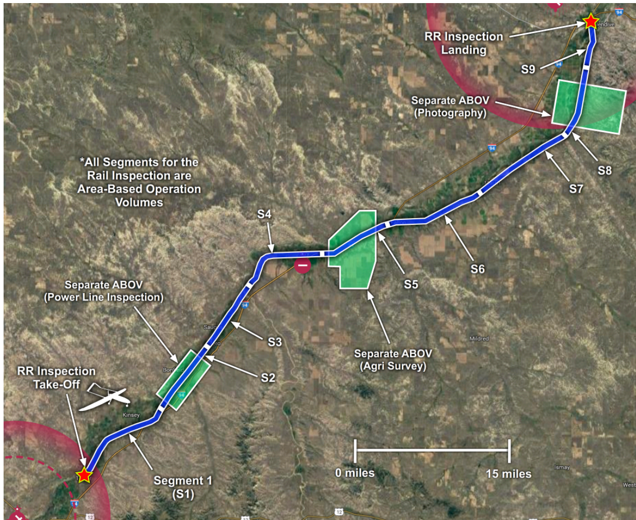
Figure 4. Rail Inspection Overview
