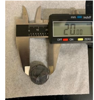
Above: First SPS Mo-dUN specimen, ~10 mm in diameter by 12.7 mm long
