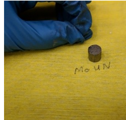
Above: First SPS Mo-dUN specimen, ~10 mm in diameter by 12.7 mm long
