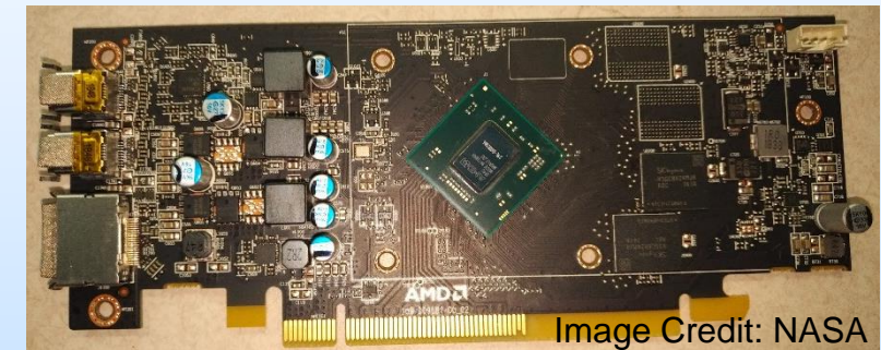
AMD e9173 Discrete GPU (14nm Global) Board without heatsink and cold plate adapter
