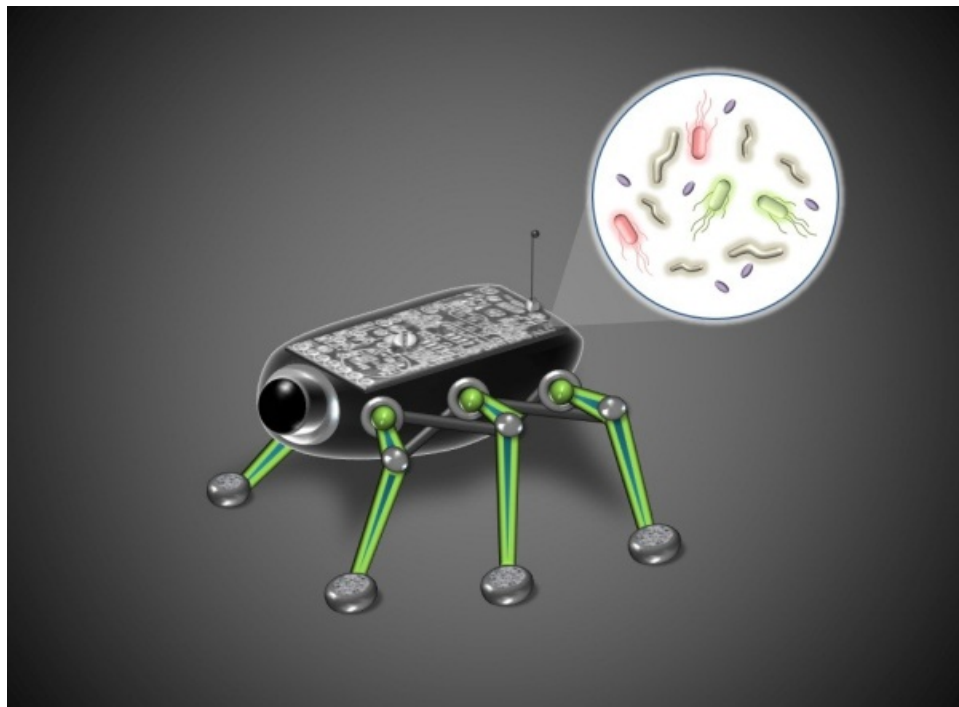
Figure 27 – A theoretical concept of a microbial fuel cell powered microrobotic system (Credit: K. Reilly/NASA NIAC).
