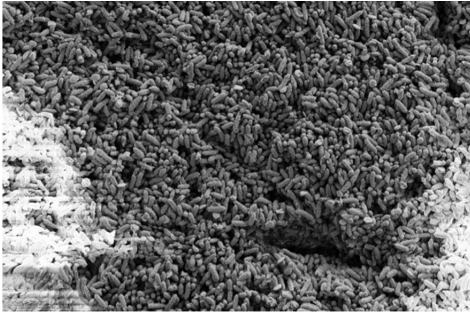
Figure 7 – a) A microscope view of an anode coated with Geobacter sulfurreducens microbe used in the Phase I study.
