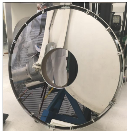
Figure 1. ES-MCAT's primary mirror in the lab at ZeCoat Corporation. The new, enhanced, protected silver coating is both more environmentally durable and more reflective throughout visible-bands (>95% average reflectivity).
