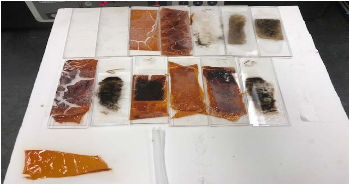
The test panel with all the sample configurations for 460C/1hr testing
