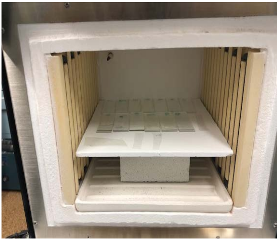
The test panel with all the sample configurations for 460C/1hr testing
