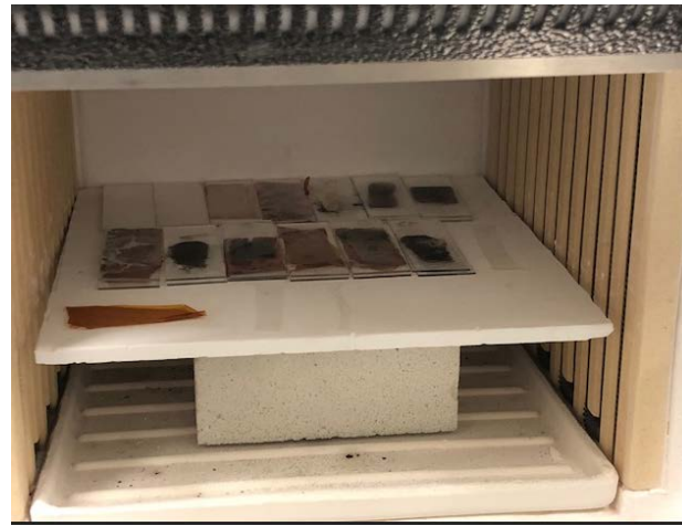
The test panel with all the sample configurations for 460C/1hr testing
