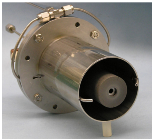
Figure 2. The JPL-designed high-current \text{LaB}_6 hollow cathode used during this campaign. The tubes at the 3 and 9 o'clock positions near the exit orifice of the cathode are the external gas injectors.
