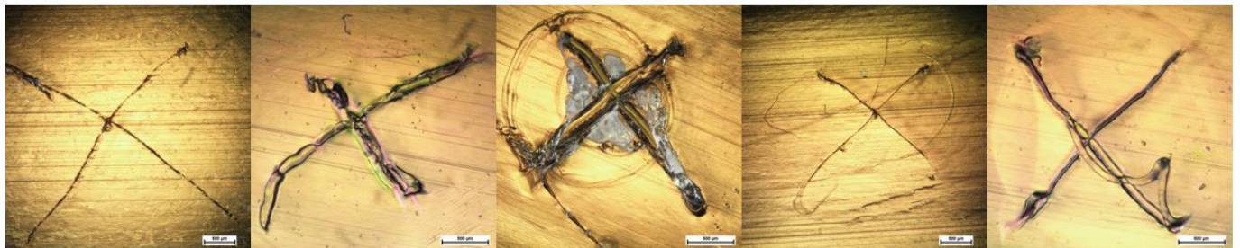
Figure 4: (From left to right) No solvent, amyl acetate, acetone IPA and MEK..
