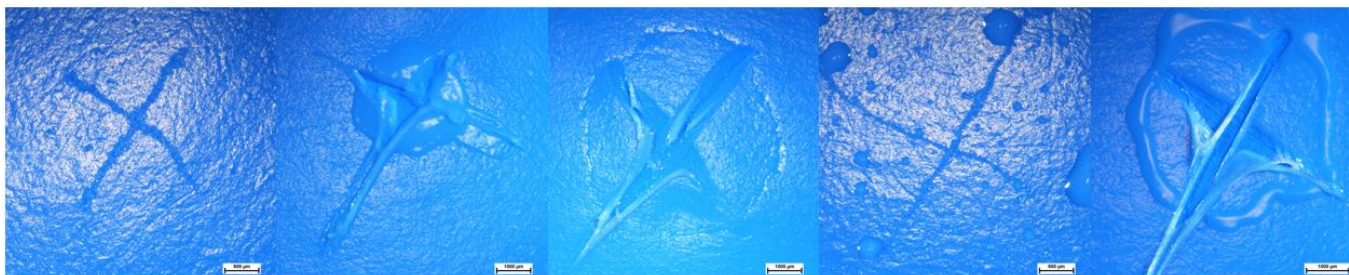
Figure 2: (From left to right) No solvent, amyl acetate, acetone IPA and MEK.
