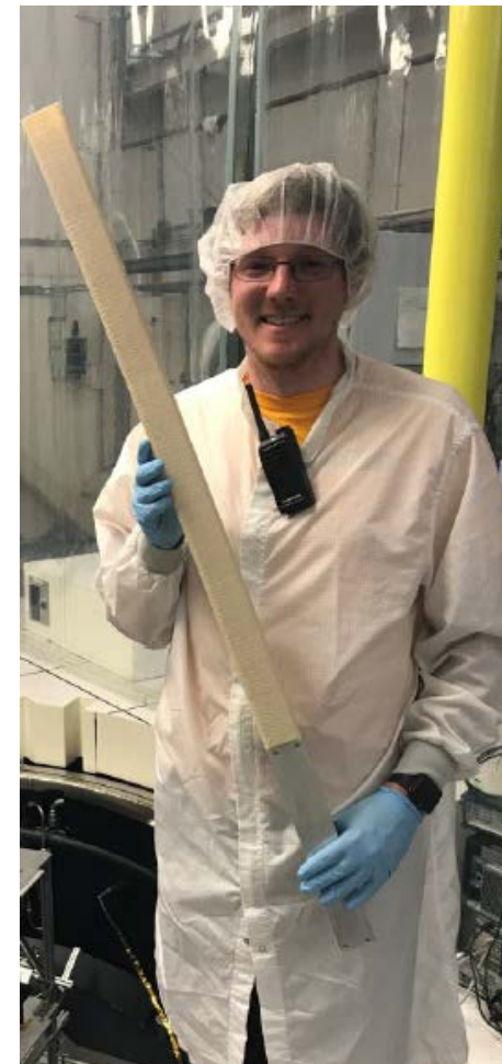
MIS Mechanical Engineer DeeJay Riley with 850 mm Beam printed in a TVAC chamber
