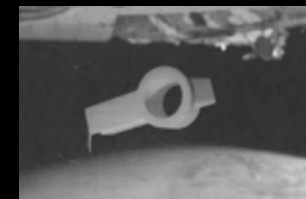
Oxygen Generation System (OGS) Adapter attaches over air inlet to obtain a consistent and accurate reading of airflow. Printed on 7/19/2016
