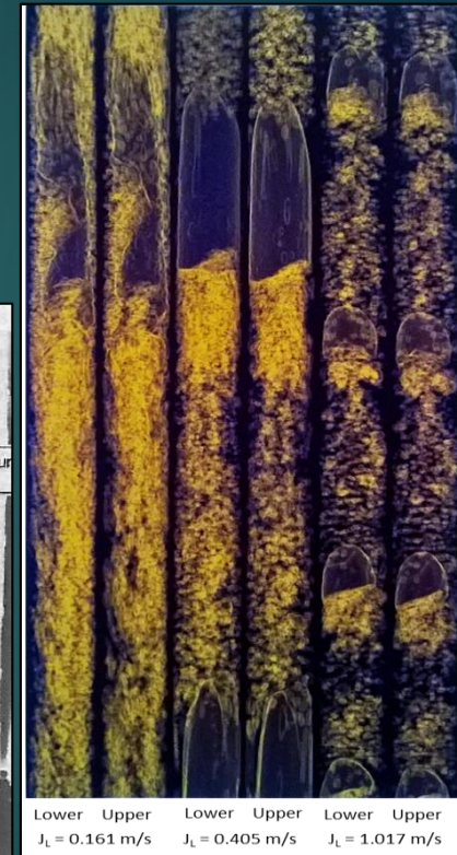
Virtual three dimensional plots of two phase flow obtained using X-ray CT. (Source: Reference 3)
