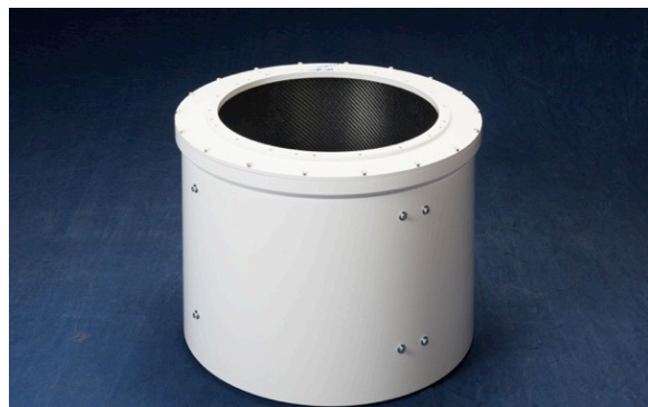
(d) Assembled Liner Holder Spool with Core Installed
