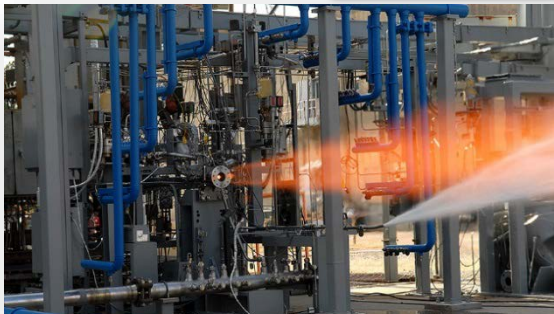
GRCop-84 AM Chamber Accumulated 2365 sec hot-fire time at full power with no issues
