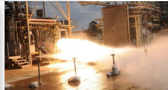
Ox-Rich Staged Combustion Subscale Main Injector Testing of 3D-Printed Faceplate
