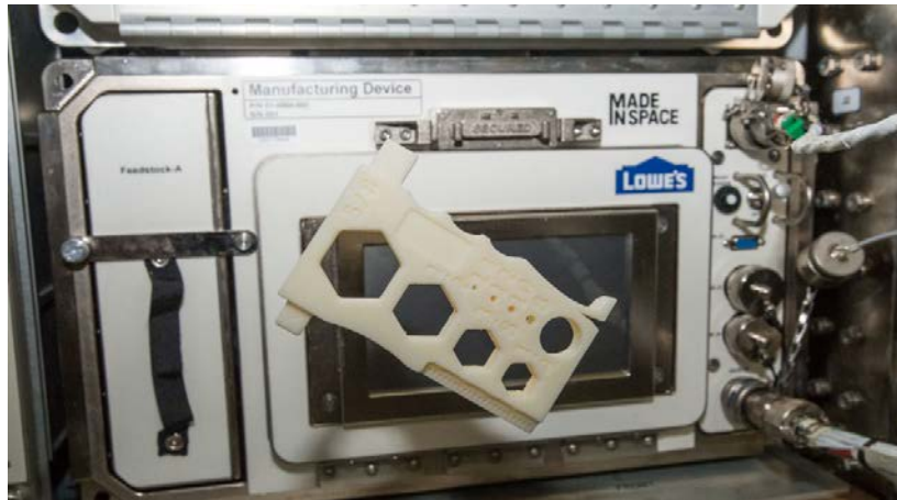
AMF on ISS with printed multi-purpose tool floating in front (photos courtesy of MIS)
