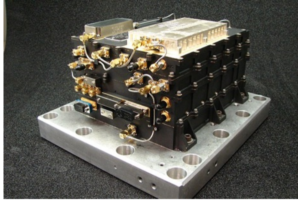
Figure 58: Electra Transceiver mass of 4.9Kg, size of 17.2cm (W) x 21.9cm (L) x 14.0cm (H) used aboard the Mars Reconnaissance Orbiter (MRO). Image Credit: NASA/JPL-Caltech.
