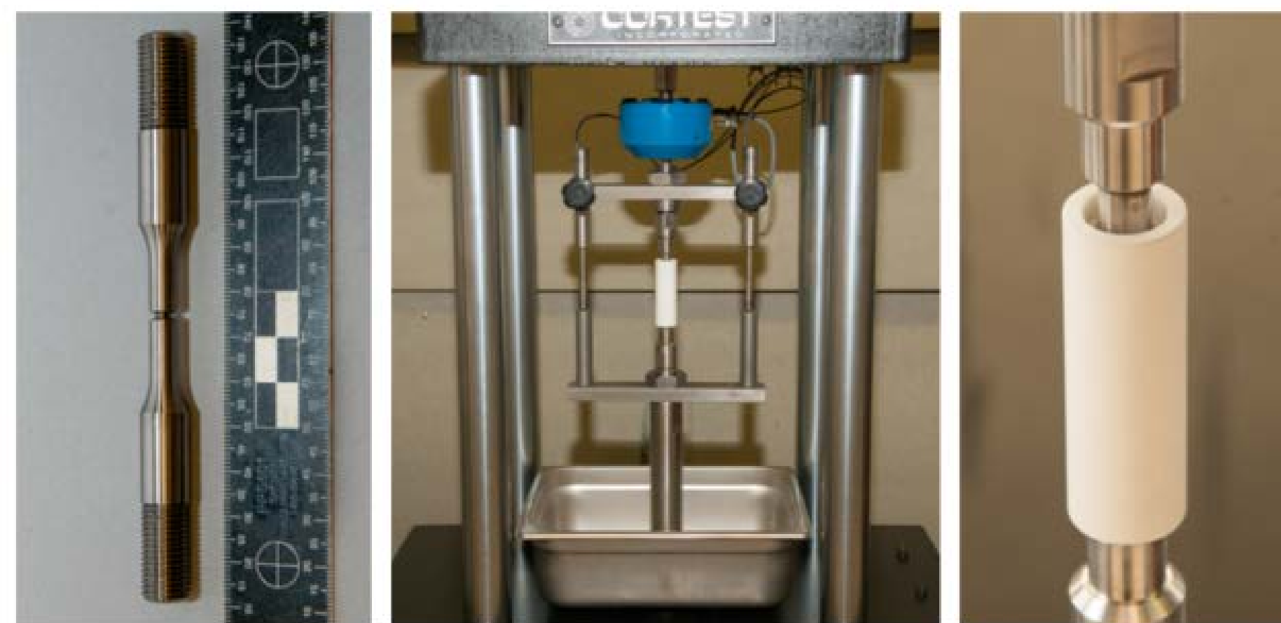
Photos: Pre-test specimen (wstf2018e20280), slow strain rate test in progress (wstf2018e20273), PTFE environmental chamber designed and used for oxidizer exposure (wstf2018e20277)
