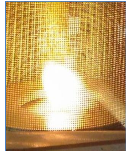
LMP-103S at atmospheric pressure.
